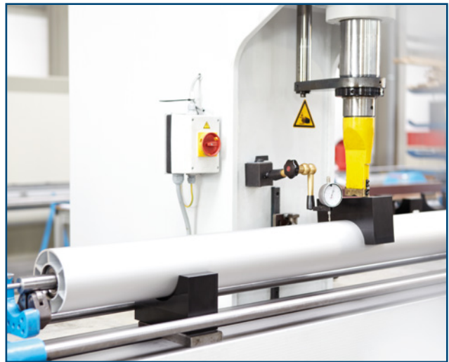
Precision straightening of technical rollers.
